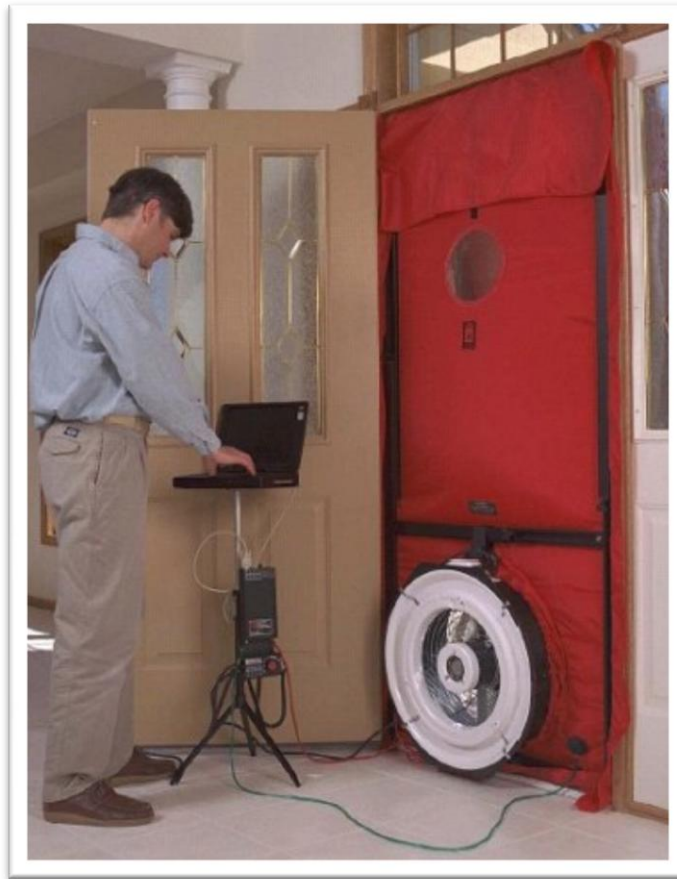
Obr. 7 Blower door – aparatura (Zdroj: Unity College Passive House, cit. 9. 8. 2012)
