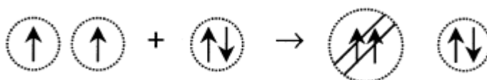
Fig. 2: A reaction between parallel electrons of oxygen and electrons of any stable compound cannot proceed due to a spin restriction (Fridovich 1999).
