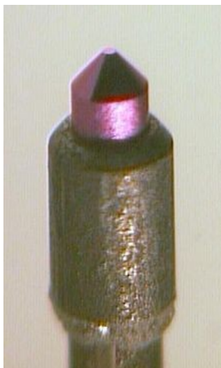
Obr. 27: Katoda z hexaboridu lanthanu ( \text{LaB}_6 ) [87]
