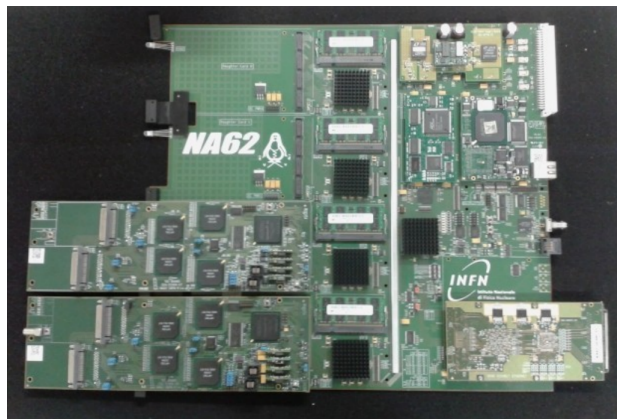
Figure 3.1: A TEL62 board equipped with two TDC boards and the quad gigabit board [3].
