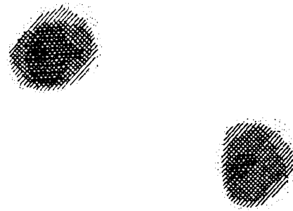
Figure 2. The first MRI image – famous Lauterbur zeugmatogram adopted from the Ref. 7. It depicts the 2D map of the proton concentration in a sample consisting of two water-containing capillaries placed in a standard 5 mm NMR tube.
