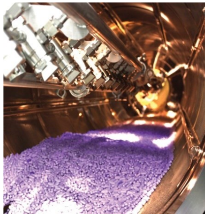
Obr. 21: Fastcoat™ Continuous Tablet Coating Systems (1 200 kg) O'Hara Technologies (pohled do bubnu) 29
