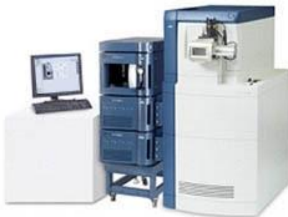
Obr.č.13 Waters nanoACQUITY UPLC™ System - Waters Micromass Q-ToF Premier™ Mass Spectrometer
