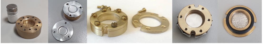
Figure 2.3: Air-tight sample holder (left) and suspension holder (very right) for Mössbauer spectroscopy experiments in the whole temperature range provided by the spectrometers. The sample stability during the experiment was tested down to 4.2 K and theoretically can reach up to a melting point of the indium seal or temperature limit of the installed temperature probe.
