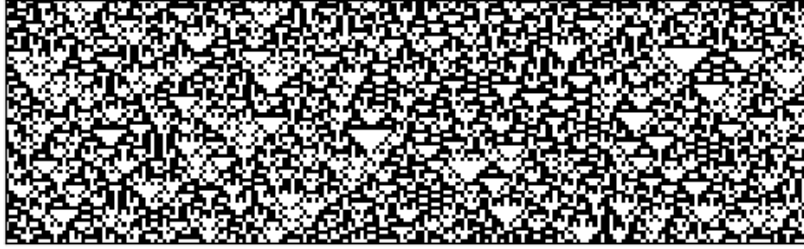
Figure 1.1: Space-time diagram of ECA 90 operating on a finite cyclic grid of 100. We typically identify the state 0 with white and state 1 with black colour. Each row of the depicted diagram corresponds with a configuration in the ECA's trajectory; thus, time is “progressing downwards”.
